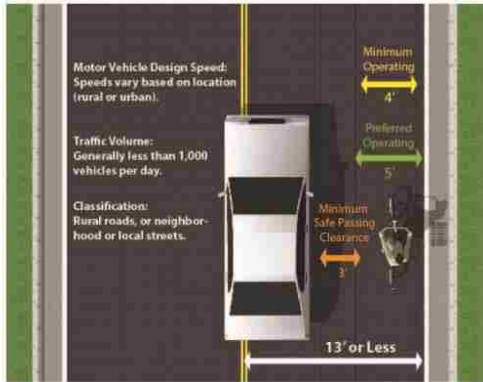
Figure 2-1: Shared lane (no special provisions) (MMMPO 2015).
