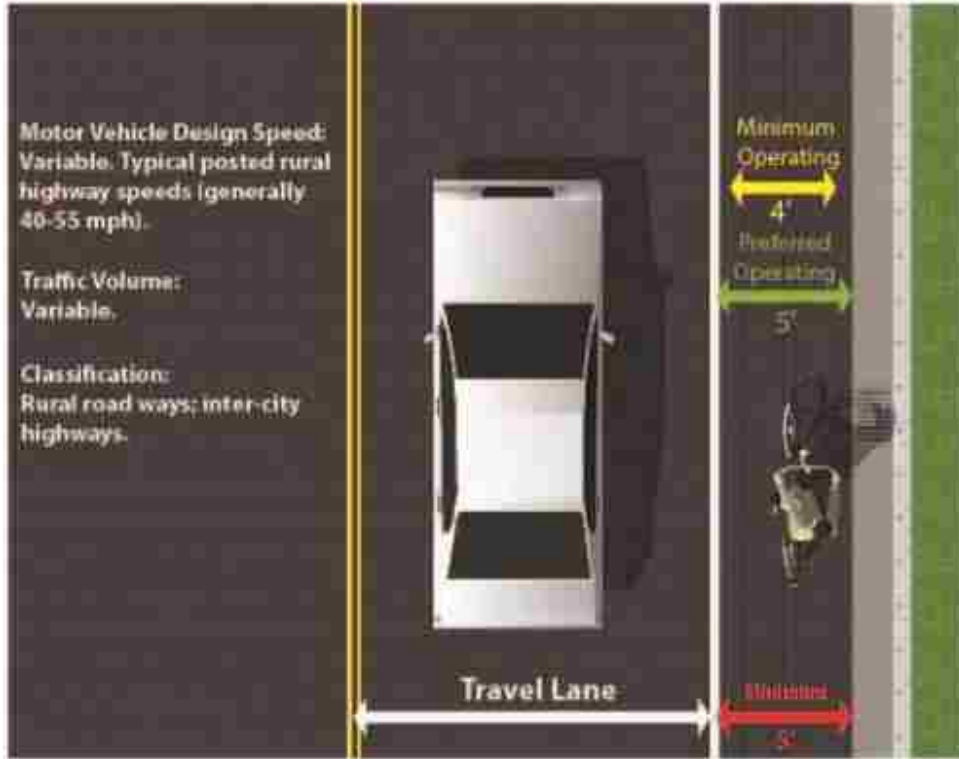
Figure 2-4: Paved shoulder (MMMPO 2015).
